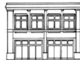
Façade articulation is improved by providing a building base and three- dimensional horizontal and vertical expression lines
